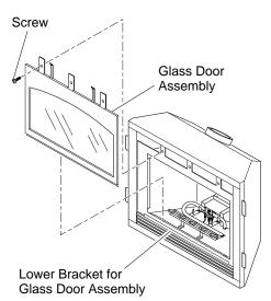
Figure 47 - Removing/Replacing Glass Door
